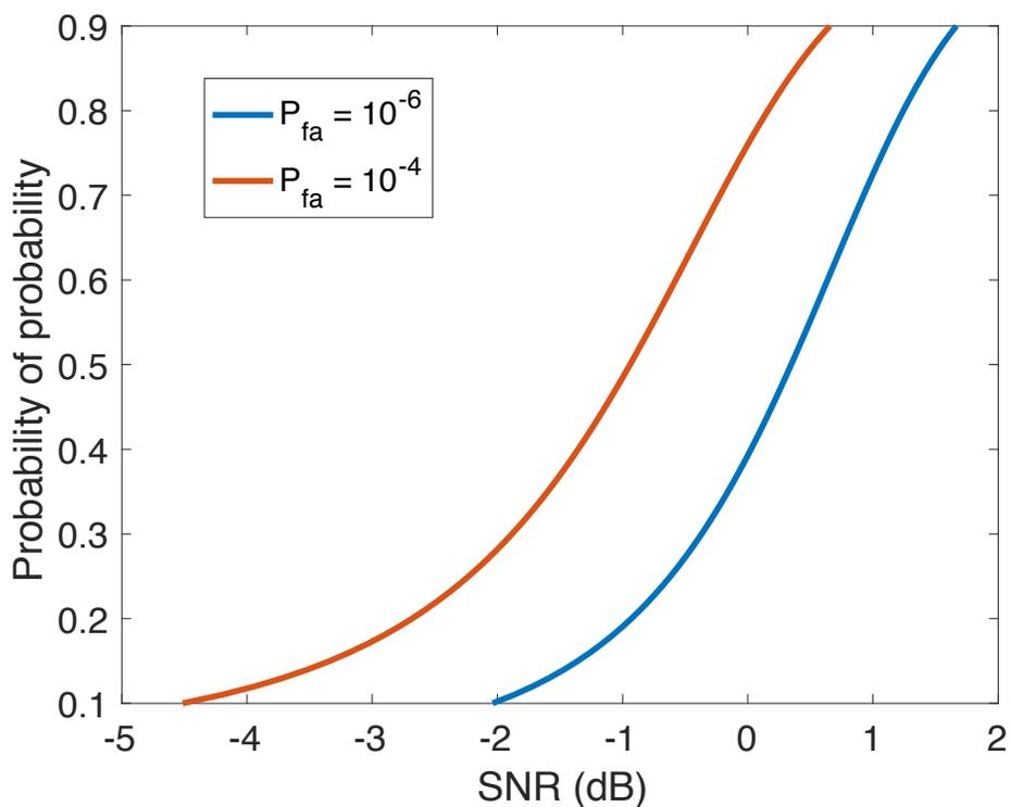
Figure 1: Probability of detection  $P_d$  vs. SNR (dB) for probability of false alarm  $P_{fa}$
